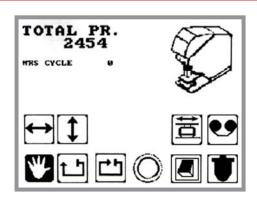
Easy touch control pad allows the operator to adjust parameters such as print speed, cliché pause, single or continuous cycle, manual mode, increase/ decrease stroke on cliché and part.
