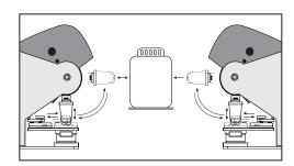
Use two printers for horizontal in-line printing both sides at one time.
