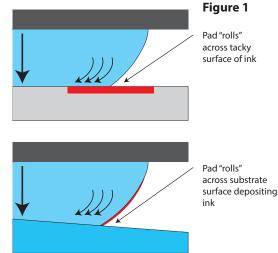
In order to achieve a satisfactory print, the pad surface must roll onto the cliché (plate) and the image area of the substrate, as shown in Figure 1.
