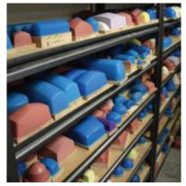
Each of these shapes could have either curved or flat printing surfaces, depending on the nature of the part to be printed. But regardless of what shape the pad has, it must roll onto both the cliché and substrate for good printing results. Try to avoid flat-bottomed pads, as they have a tendency to trap air when they come in contact with the cliché, hampering ink pickup. Again, the more rolling action that is achieved, the more ink that will be transferred.
