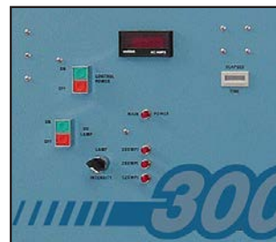
▲ Power panel controls lamp duration counter, power regulator and on/off switches
