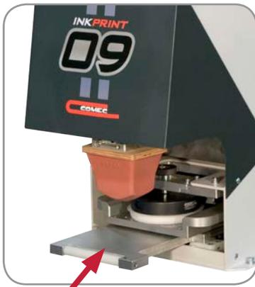
**KV09 programmable pad cleaning tray located under cliché.**
