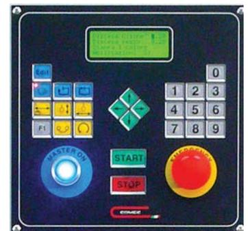
▲ **Easy touch pad controls** have many programmable features such as pause, speed and timing sequence.
